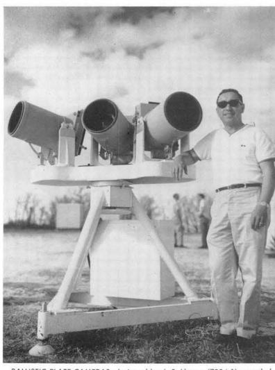
BALLISTIC PLATE CAMERAS, designed by J. S. Llamas (7224-1) recorded the RFD-1 reentry as broken streaks on 8x10-in. glass film plates. Mr. Llamas engineered the conversion of the three surplus aerial mapping cameras and associated newly-designed features for the RFD-1 flight.
